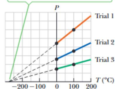
Pressure versus temperature for experimental trials in which gases have different pressures in a constant-volume gas thermometer
